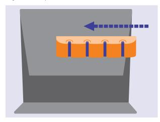
Check that the ejection blocks in the gap of the magnet are attached before placing the MACS Column into the magnetic field of the QuadroMACS Separator. Do not remove ejection blocks of the QuadroMACS Separator.
