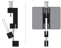
Insert Adapter for MS, LS and LD Columns in the magnetic field of SuperMACS™ II Separator (for details, see "SuperMACS II data sheets"). Place the M Column in the Column Adapter and the 13 mL collection tube in the lower tube holder.
