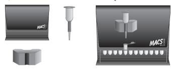
Attach MiniMACS™ or OctoMACS™ Separator to the MultiStand and place M Column in the separator. Place a collection tube under the M Column.
