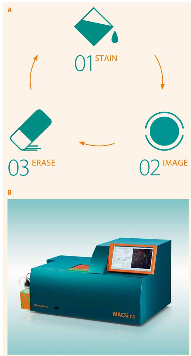
**Figure 1:** Schematic of the MICS principle (A) and MACSima Imaging Platform (B). The MACSima Imaging System performs the three steps of MICS technology in a fully automated manner: 1) The sample is stained, 2) imaged, and 3) the signal erased. After a cycle is completed, the process automatically continues with the next cycle, enabling the analysis of hundreds of markers on a single sample.
