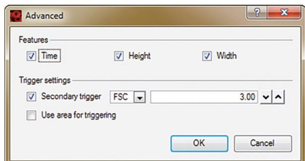
**Figure 1:** The parameter **Height** must be activated for analysis of ploidy levels. Optionally, **Width** can also be activated.
