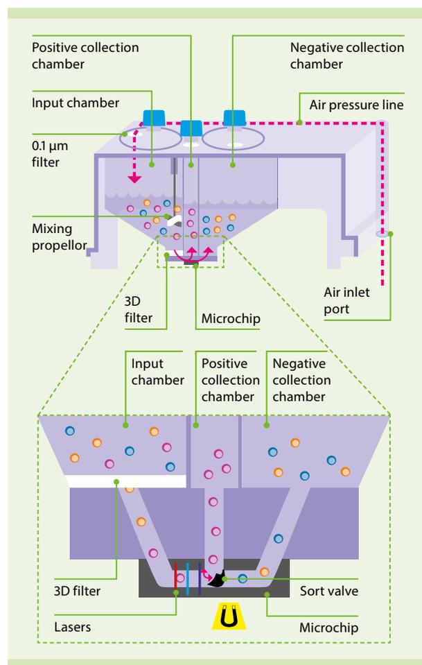
**Figure 1: The sorting mechanism of the MACSQuant Tyto.**
