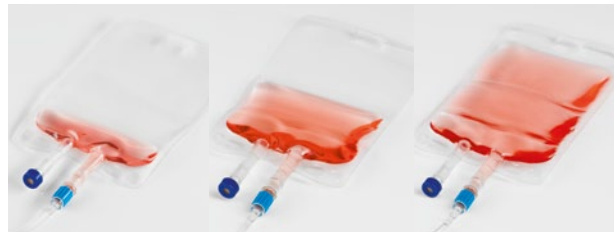
Figure 8: Consecutive filling of the compartments of the MACS GMP Cell Expansion Bag.
