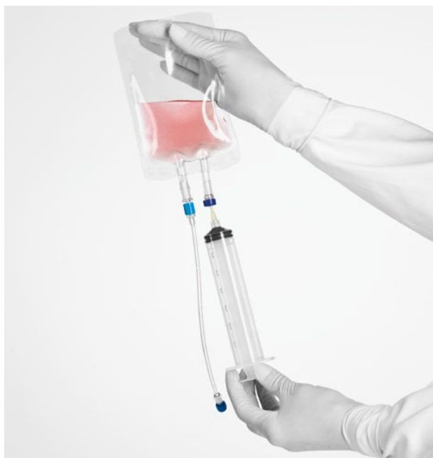
Figure 17: Empty syringe attached to septum port of a MACS GMP Cell Culture Bag.
