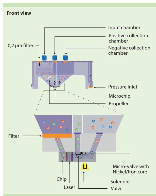
**Figure 1: The sorting mechanism of the MACSQuant Tyto.**
