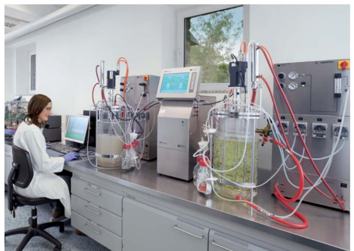
Bioreactor for production of high-quality recombinant proteins.
